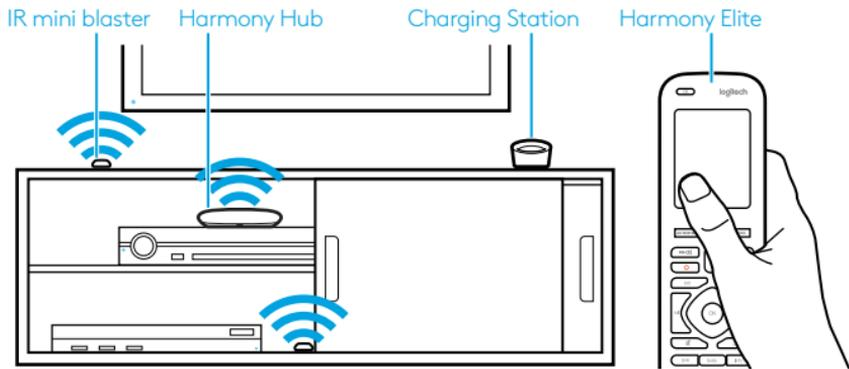
The Harmony Hub can be placed in any unobstructed location where IR signals can be transmitted to AV equipment or it can be placed behind closed cabinets with the IR mini blaster transmitters connected to the hub and positioned as shown above.
